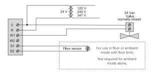
Connection layout for a hot water valve
