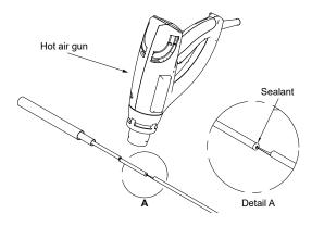
2.6 Insert the 6 x 40 mm heat shrink tube into one of the 65 mm (2 9/16") cut wires.
