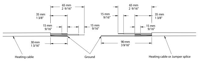
2.3 Insert the 6 x 40 mm into the earlier ground section cut at 90 mm (3 9/16").
