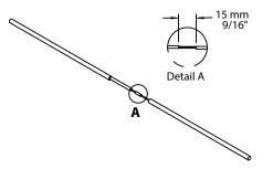
2.8 Insert the 6 x 40 mm heat shrink tube over the connection and make sure it is centered to the mechanical connection. Then heat the entire length of the tube with a hot air gun (do not overheat it), make sure the tube has shrunk enough to see the sealant coming out of both sides.
