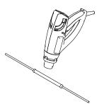
3.2 Then insert the 18 x 155 mm tube over the 12 x 110 mm tube and center it well and heat the heat shrink tube along its entire length with a hot air gun (do not overheat it), make sure the tube has shrunk enough to see the sealant coming out of both sides.
