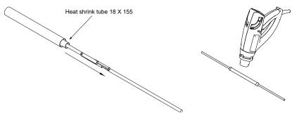
3.3 Repeat the same steps 2.3 to 3.2 for connecting the other extremity of the jumper splice.
