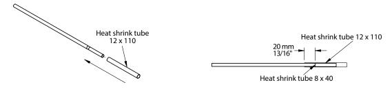
5.6 Heat the entire length of the heat shrink tube with a hot air gun (do not overheat it) and while the tube is still hot, gently crush the end of the tube over 7 mm (5/16") with electrician's pliers until the heat shrink tube is cold. The tube must remain visibly sealed when the pliers are removed. If the tube does not remain sealed, repeat this step.
