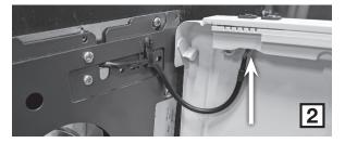
3. Using a screwdriver, press the plastic tab on both sides of the integrated thermostat and remove it (Figure 3).
