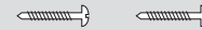
2 Screws (1-1/2") with a 1/4" (6.5 mm) diameter head minimum, suitable for securing the back box directly to a stud.
