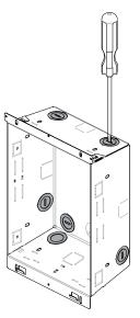
ATTENTION: Be sure to push in the right hole by placing the back box in the correct direction. The notches will be positioned at the bottom [A], or at the right [B].
