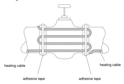
Installation of heating cables on valves by means of a wire guard for a quick disassembly and re-assembly of the heating during maintenance work at the valve.
