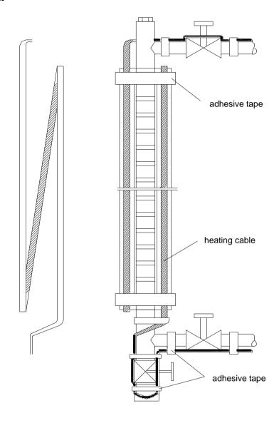
Remark: Attach heating cable with self-adhesive aluminum tape.
