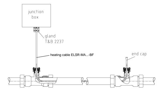
If no potable water requirements apply, end cap may be inserted downstream in pipe.
