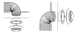
2.7 Push the pipe completely back into the structure and attach the collar to the ceiling or wall. Then attach the diffuser to its collar.
