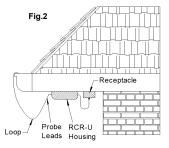
Fig.3 Sensor Wire Application with Gutter
